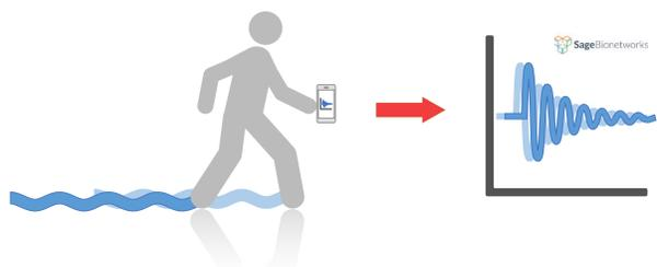
2. Waveforms are processed using various methods, such as **smoothing** and **Fourier transforms**, in order to reduce data into simpler representations for comparison.
